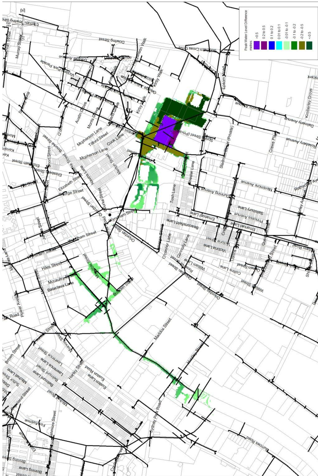
Figure F2 Layout 100 Year ARI Peak Water Level Difference for FM1 Less Existing
